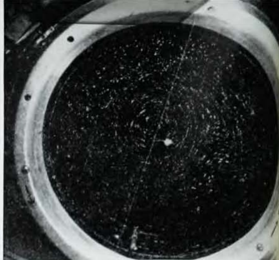
Fig. 4. Low-rotation streak-flash photograph of fluid motion induced in a rotating cylinder heated at the perimeter and demonstrating a rather symmetrical vortex. This type of flow is sometimes associated with flow patterns which are observed in the free atmosphere in the tropical regions. Note the absence of pronounced wavelike disturbances. (Cylinder rotation rate is 2.92 rpm.)
