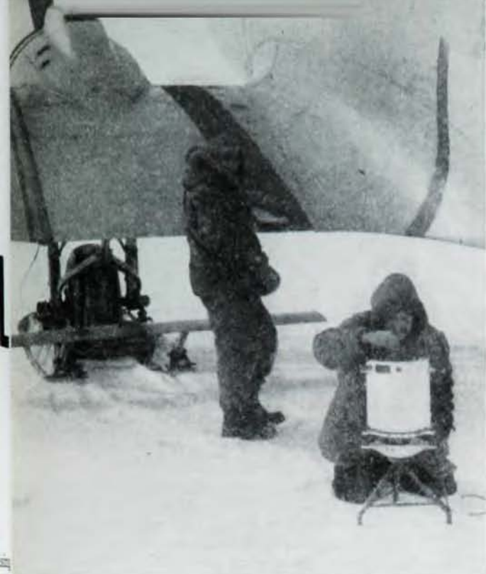
Fig. 2. Reading the portable gravity meter on the Arctic ice pack north of Alaska during an aircraft landing for scientific observations.
