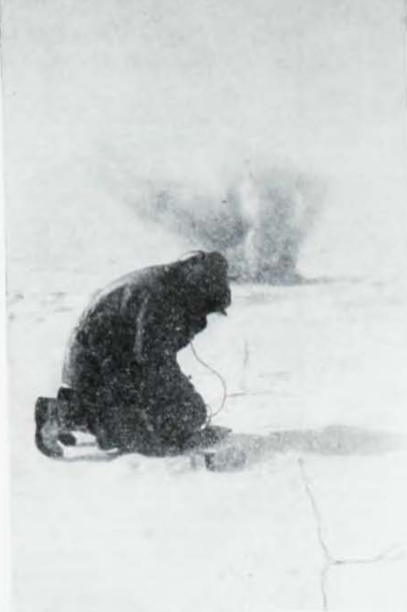
Fig. 1. Setting of powder charge on the Arctic ice pack during measurements of ocean depth.
