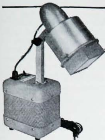
Hanovia Utility Model Quartz Lamp—high-pressure, quartz mercury arc lamp. Wavelengths of 3130 angstrom units and shorter.
