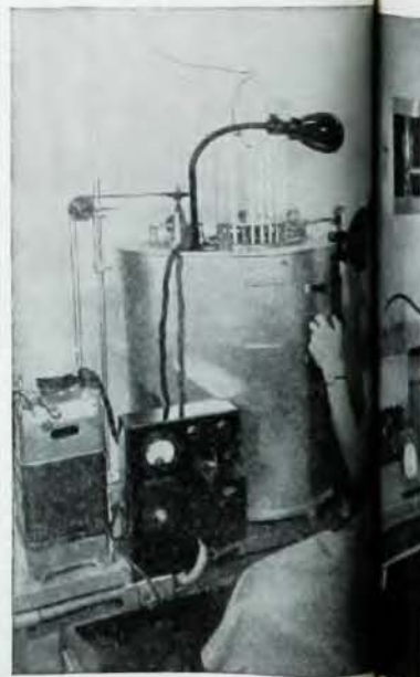
Fig. 2. Liquid-in-glass thermometers are shown being tested at the National Bureau of Standards by comparison with one of the Bureau's standard platinum resistance thermometers. For the temperature range from 0° to 100°C, the thermometers are immersed in a mechanically stirred water bath. The power input to the heater is controlled by the variable transformer at the left of the bath. The thermometers under test are read with a telescope, and the corresponding reading for the platinum-resistance thermometer is obtained with a Mueller thermometer bridge.
