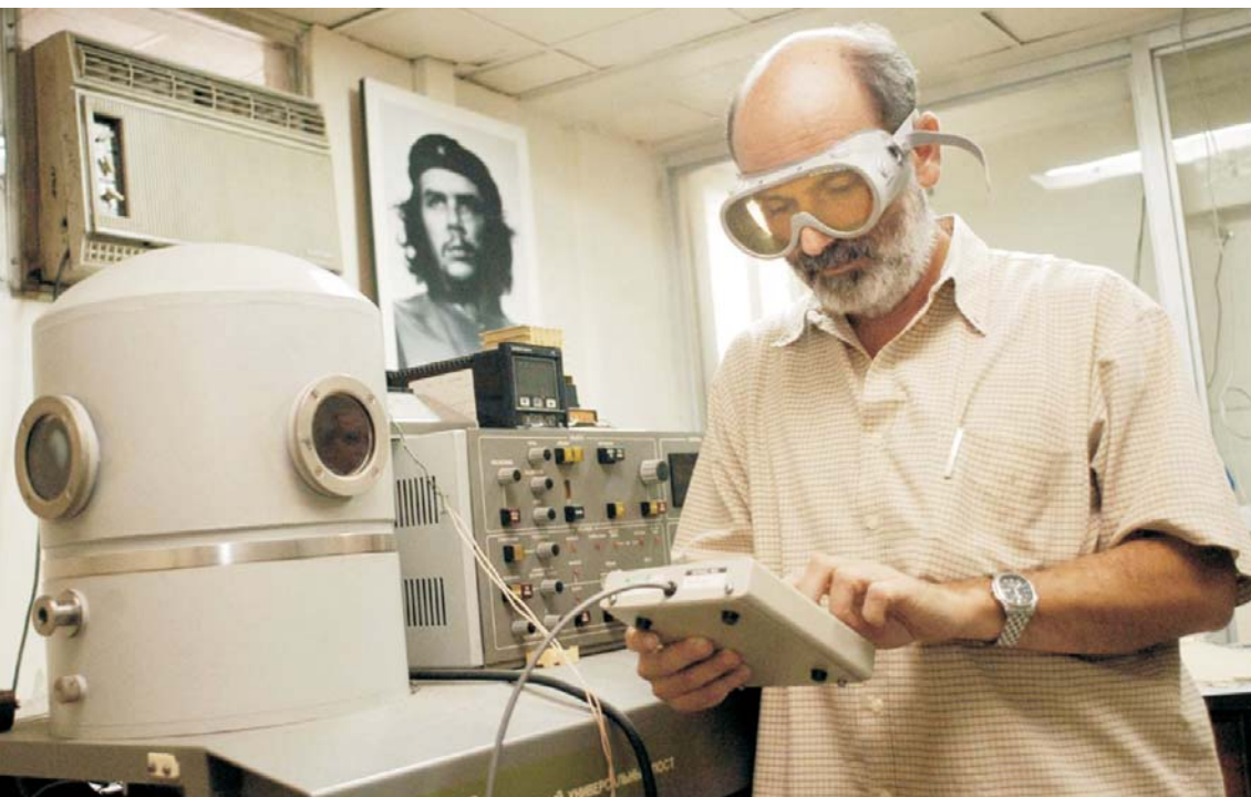
Figure 1. A pulsed laser deposition system in the Institute of Materials and Reagents (IMRE) of the University of Havana. IMRE was established in 1985 to support industrial needs for materials, chemicals, lasers, and optoelectronics. This system allows laser deposition and in situ studies of high- T_c superconductors, manganites with colossal magnetoresistance, and other thin-film oxides.
