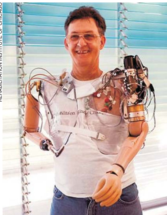
Electrodes on one side of double-amputee Jesse Sullivan's chest pick up thought-generated signals from his nerves to control a state-of-the-art prosthetic arm. His other arm is an old-fashioned pincer.
