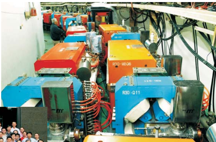
Two rings of magnets (above) store particles and crisscross to form interaction areas in the upgraded Beijing Electron-Positron Collider. In June, scientists from China, the US, and elsewhere met in Beijing to discuss collaborations in high-energy physics.
