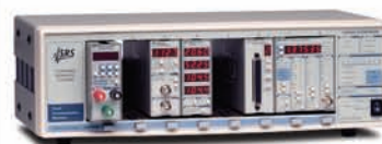
SIM900 Mainframe loaded with a variety of SIM modules
