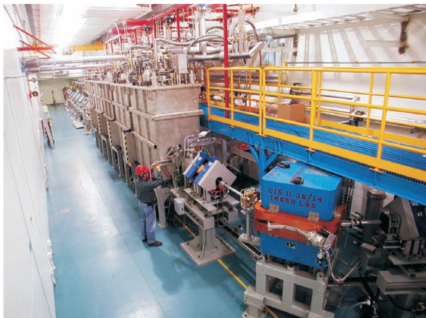
The superconducting linac at TRIUMF's upgraded radioactive isotope accelerator was successfully tested in April. The five cryomodules (large off-white blocks) house 20 RF cavities. The beamline to the experimental hall is visible in the distance.
