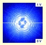
and oxygen. In a TEM, most of the electrons pass through the thin electron-transparent sample without scattering; those that are scattered have their phase shifted. Scattered and unscattered electron waves are then focused and recombined into an image. Unfortunately, for weak-
