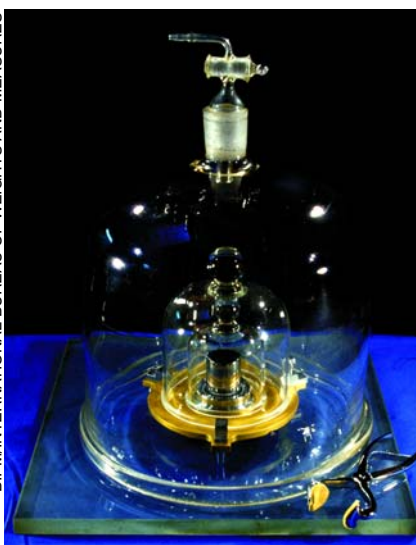
The international prototype of the kilogram is 39 mm in diameter and 39 mm high. This is a copy of the actual reference standard.
