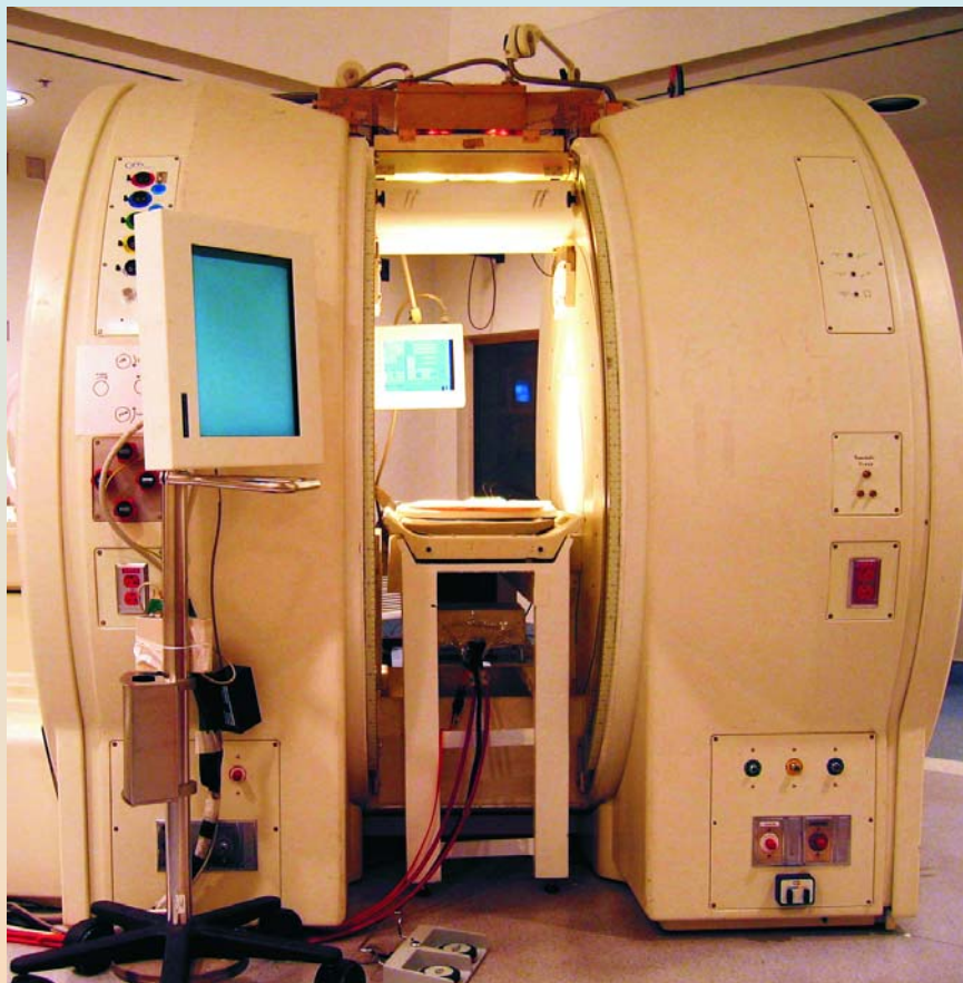
Stanford's hybrid XMR system consists of two doughnut-shaped coils that generate the magnetic resonance field. The x-ray detector (connected to red and black cables) lies below the patient table. Above the table and spanning the gap between the doughnuts is the housing for the x-ray tube. (Courtesy of Arundhuti Ganguly.)
