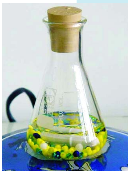
Figure 2. A metal bar, controlled electromagnetically, forces crystals between glass beads and breaks them up. At the same time, new crystals form. Eventually chiral purity results. (Courtesy of C. Viedma.)
