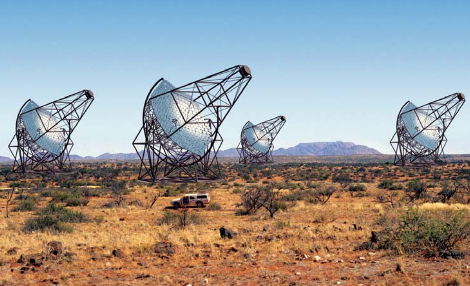
Figure 2. The four Cherenkov telescopes of the recently completed HESS facility sitting at an altitude of 1.8 km in Namibia's Khoma Highland. Each telescope's segmented 13-meter-diameter parabolic reflector directs the flash of Cherenkov light from an incident high-energy cosmic-ray shower onto the focal-plane array of phototubes that serves as its high-speed camera. (Courtesy of the HESS collaboration.)
