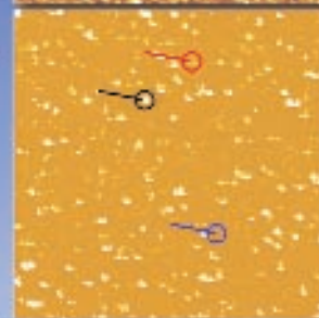
Right: Topography and current images at a bias of 1.5 volts, 50pA scale, 2μm scan. Measured IV curves are shown from marked areas on the second image. Samples courtesy of Kannan Krishnan Lab, Univ. of Washington.
