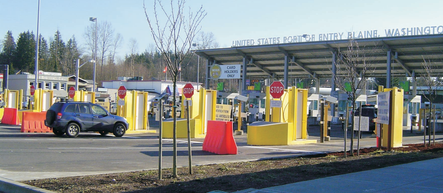
Figure 1. Highly sensitive portal monitors (yellow) installed in passenger lanes at the Pacific Highway crossing in Blaine, Washington, can detect the presence of small amounts of radioactive material just meters away. False alarms occur somewhat frequently—most often from naturally radioactive agricultural products, ceramic tiles, and the rare passenger who may have just received a thallium, technetium, or iodine injection from a physician.
