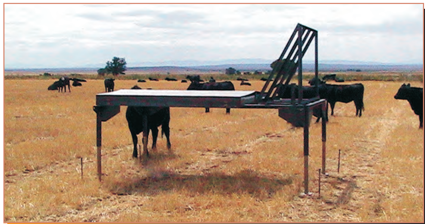
Solar-powered scintillators for the Telescope Array will sit on platforms scattered around the central Utah desert.
