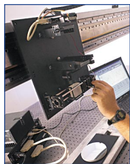
Long Trace Profilometer Perform absolute figure measurements on large flats, spheres and aspheres
