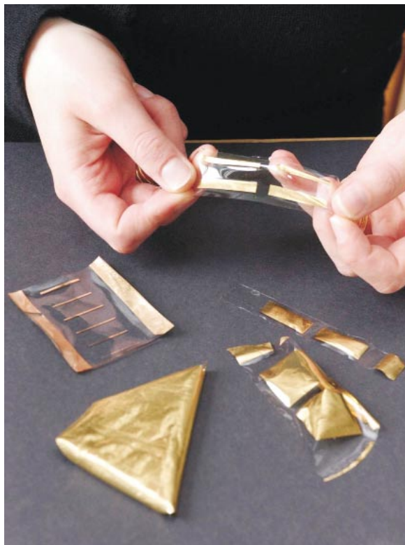
Figure 1. Stéphanie Lacour demonstrates the flexibility of the stretchable conductor she developed with Princeton University's Sigurd Wagner, Zhenyu Huang, and Zhigang Suo. (Courtesy of Lacour.)
