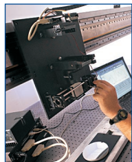
Long Trace Profilometer Perform absolute figure measurements on large flats, spheres and aspheres
