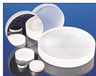
Specular Reflectance Standards Measure surfaces with low or high specular reflectance values
