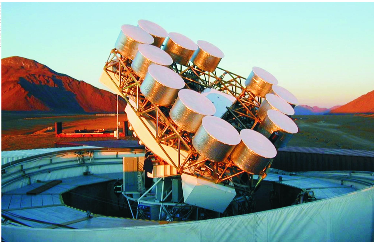
FIGURE 2. THE COSMIC BACKGROUND IMAGER, sitting on an arid plateau high in the Chilean Andes, is an interferometric array of 13 separate radio antennas mounted on a 6 m tracking platform. Each antenna is a 90-cm-wide parabolic reflector enclosed in an aluminum shield can with a teflon cover transparent to microwave radiation.
