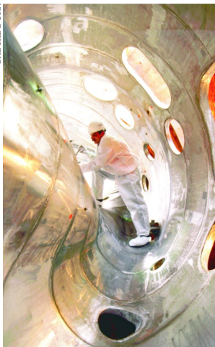
THE PLASMA VESSEL will be adapted to match the plasma shape in Wendelstein 7-X, a quasi-poloidally symmetric stellarator under construction in Greifswald, Germany. This prototype is to scale.
