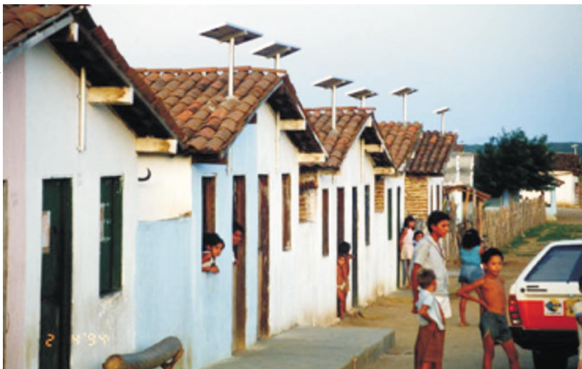
FIGURE 3. IN THE VILLAGE OF CACIMBAS in Brazil's Ceara state, 50-watt photovoltaic systems provide homes with electricity for fluorescent lighting. With support from the US Department of Energy, the Brazilian energy ministry is installing such systems in several states in the Amazon region and the country's northeast.
