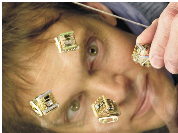
RESEARCHER DOUG ADKINS inspects a group of tiny robots he and colleague Ed Heller are developing at Sandia. The robots are intelligent and communicate with each other.
