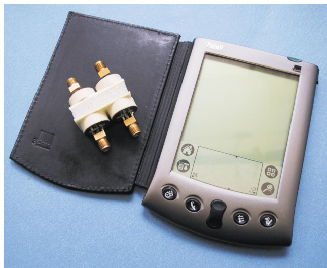
FIGURE 5. COMPACT ANTENNA ARRAY. This prototype array contains four antennas and has an overall size of less than a third of a wavelength. Despite the small size of the array, the individual antennas operate independently due to their directional diversity: In essence, each of these antennas “looks” in a different direction. Such compact antenna arrays may be useful for achieving high information transfer rates in small wireless devices. In a sufficiently rich scattering environment (such as indoors, or in a city), transmission between two sets of these compact antennas can achieve an information transfer rate almost four times larger than single-antenna to single-antenna transmission.
