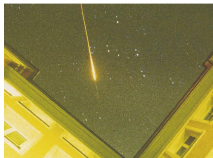
FIGURE 1. SELF-CHANNELED white light pulse pushes through the atmosphere above a courtyard at the Friedrich Schiller University in Jena, Germany. The beam was launched from the courtyard. (Courtesy of Ludger Wöste.)
