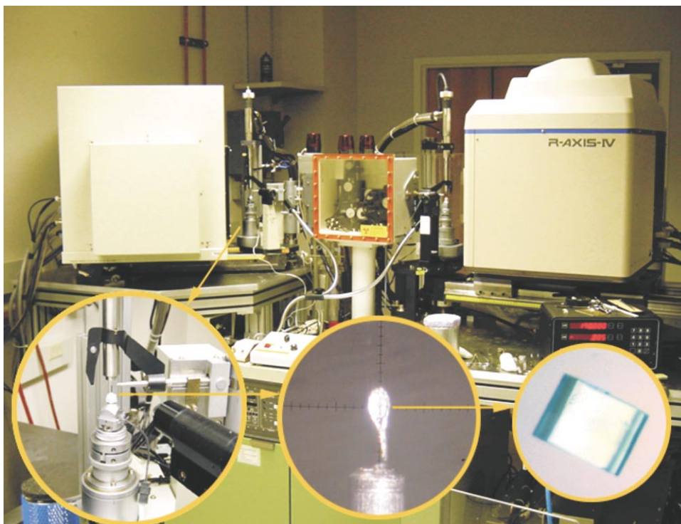
FIGURE 1. TYPICAL INSTRUMENTATION used for measuring x-ray diffraction of macromolecular crystals. The large image shows two x-ray detectors (large boxes on the left and right of the image) and two goniometers. The inset images are progressive closeups of the setup. The left image shows the goniometer on which the crystal is positioned. The x-ray collimator (horizontal, pointing left), cooling nozzle (vertical, pointing down), and centering microscope (horizontal, pointing back) can all be seen. The black piece of metal affixed to the collimator and around the cooling nozzle is a beam stop that prevents the majority of x-rays that pass directly through the crystal from saturating the detector. The crystal is harvested from its growth environment with the fiber loop shown in the center image and plunged into liquid nitrogen for rapid cooling. The loop is then placed on the goniometer and positioned so that the crystal is centered in the x-ray beam. The rightmost image shows a typical protein crystal. (Courtesy of Brett Chevalier.)
