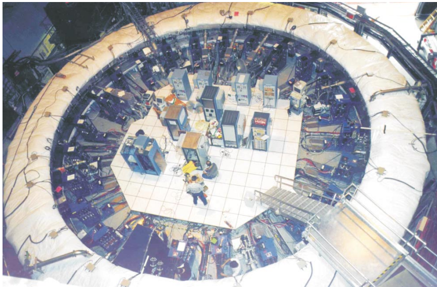
FIGURE 1. STORAGE RING of the Muon ( g - 2 ) Collaboration's experiment at Brookhaven. An iron-core superconducting magnet provides the very stable and uniform 1.45-T field that keeps the 3.1-GeV muons circulating through the ring's 9-cm-diameter vacuum pipe.
