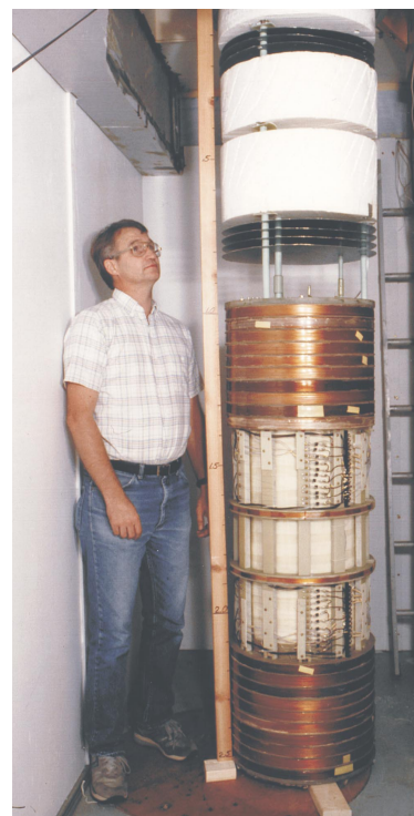
FIGURE 3. WATT-BALANCE EXPERIMENTS , which compare mechanical power to electrical power, produce the best value for the Planck constant h . In NIST's two-story-tall watt balance, the gravitational force on a mass standard is balanced by the magnetic force on a current-carrying coil in one phase of the experiment. (a) Richard Steiner positions the mass standard at the top of the watt balance. (b) Edwin Williams checks the superconducting magnet used to generate the radial magnetic field at the lower level of the watt-balance experiment.
