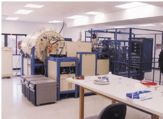
FIGURE 3. ACCELERATOR MASS SPECTROMETRY SYSTEM. This example, an NEC Model 1.5SDH-1 Pelletron, is based at the University of Georgia's Center for Applied Isotope Studies.
