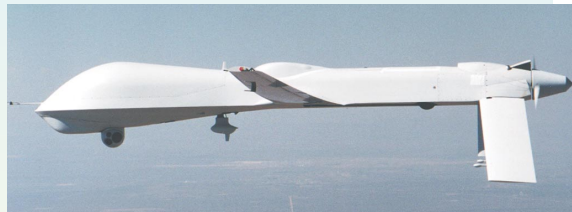
THE UNMANNED PREDATOR AIRCRAFT features synthetic aperture radar and stays airborne for up to 40 hours.
