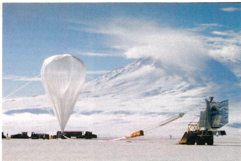
THE BOOMERANG BALLOON, minutes before launch in December 1998 from the US Antarctic base at McMurdo. By the time it reaches its 40 km cruising altitude, the balloon will have expanded a hundredfold. In the background is the active Mt. Erebus volcano.
