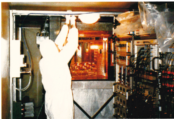
THREE SODIUM-IODIDE CRYSTALS (brass-colored cylinders) set into the shielded copper box at the Gran Sasso Laboratory, where a member of the DAMA team works on the installation. With nine such crystals to record nuclear recoils, the DAMA team found evidence for weakly interacting massive particles (WIMPs). (Photo courtesy of the Italian National Institute of Nuclear Physics.)
