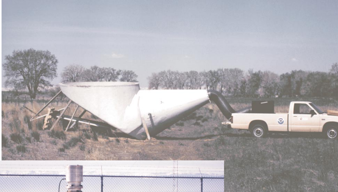
FIGURE 1. EXPERIMENTAL LOW-FREQUENCY SOUND GENERATORS are used for remote probing and propagation studies. The 10-foot-diameter horn (above) produced audible sound at 100 Hz, which was tracked with a Doppler radar to altitudes of 20 kilometers to obtain temperature profiles of the atmosphere. The 100-gallon sphere with a 1 m neck (left) is a Helmholtz resonator tunable from 10 to 50 Hz. Compressed air is released by rupturing a diaphragm, producing sound waves used for calibrating and testing infrasonic arrays.
