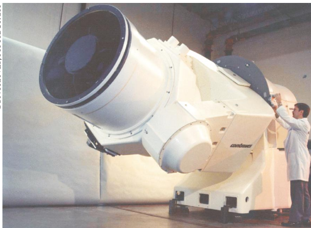
A 1-METER-APERTURE TELESCOPE of the kind deployed by the US Air Force for tracking artificial satellites. This one is still in the manufacturer’s showroom. The one on Hawaii’s Haleakala volcano was used part-time by the Jet Propulsion Laboratory’s NEAT project to search for near-Earth asteroids. “They look and move almost like naval gun turrets,” says NEAT astronomer Davis Rabinowitz, referring to the unusually rugged mounts needed for the telescopes’ rapid repointing requirements.
