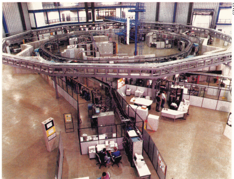
FIGURE 2. NATIONAL SYNCHROTRON LIGHT LABORATORY (LNLS) in Campinas, near São Paulo, Brazil. This facility, the first synchrotron light source in the Southern Hemisphere, has a 1.3 GeV electron storage ring and 10 beam lines providing access to photon energies from 10 eV to more than 10 keV. Active research at LNLS includes chemistry, biology, physics, and materials engineering.
