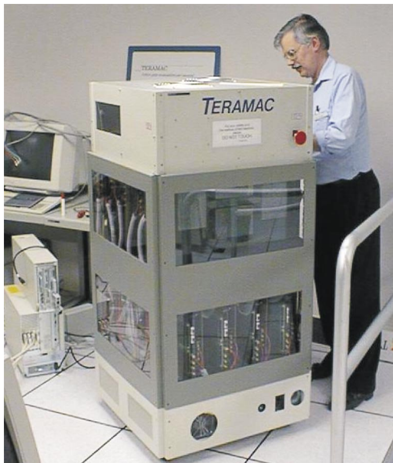
FIGURE 1. THE TERAMAC EXPERIMENTAL COMPUTER with one of its developers, Philip Kuekes. “Tera” denotes the fact that the machine performs one trillion gate operations per second (one million gates operating simultaneously at 1 megahertz); “mac” stands for “multiarchitecture computer.” Teramac, built at Hewlett-Packard Laboratories in 1995, contains over 220 000 known manufacturing defects, yet operates perfectly.
