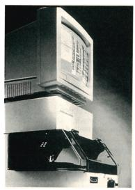
XY sample positioner and zoom optics. All three models include a color video microscope for viewing the sample surface. All scans are referenced to an optical flat to provide a stable baseline for measuring waviness, flatness, and curvature. Veeco Metrology Group, 112 Robin Hill Road, Santa Barbara, California 93117
