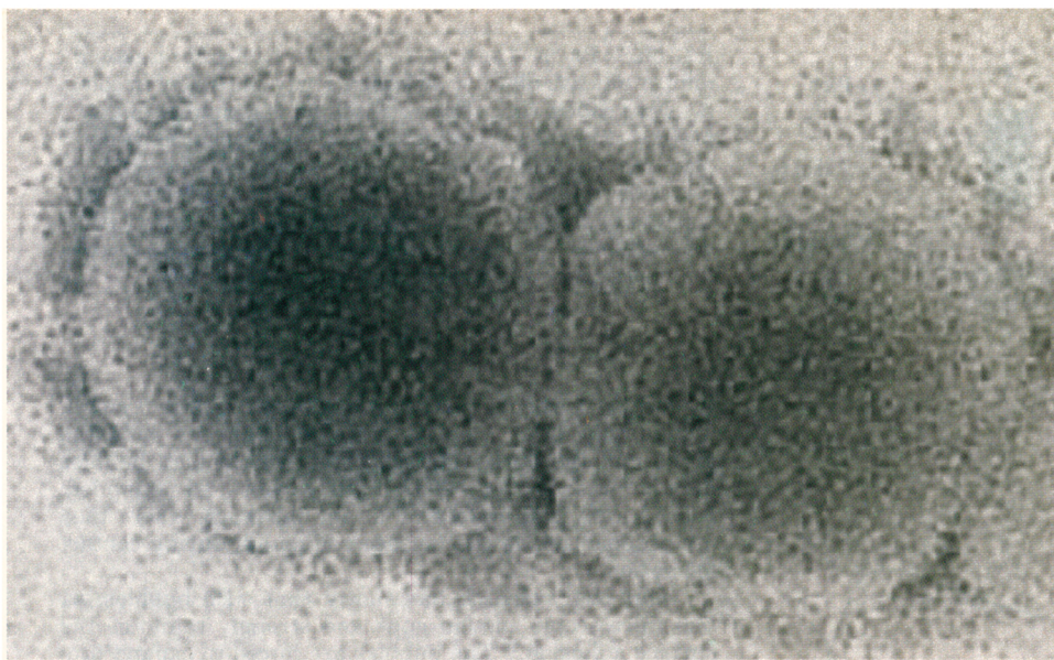
FIGURE 1. STICKY LATEX particles, 80 nm in diameter. This transmission electron micrograph shows acrylic latex particles deformed under the influence of surface forces. The softer the particles, the larger the deformation and contact area, and therefore the greater the adhesion. Controlling the stickiness of latex particles is important for film formation in many applications, including paints, varnishes, and adhesives. (Photograph courtesy of Patrick Coupard, Elf Atochem Co.)
