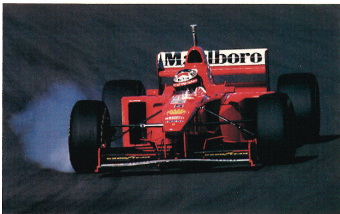
FIGURE 6. MODERN FORMULA ONE racing cars, like the Ferrari shown here, are safer than their predecessors because of the energy-absorbing composites used in their construction.
