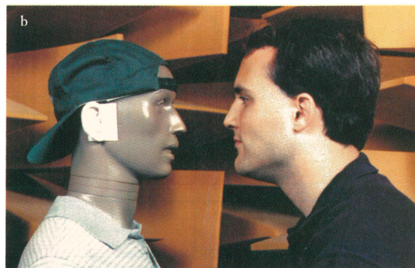
FIGURE 4. THE ANATOMICAL TRANSFER function, which incorporates the effects of secondary scatterers such as the outer ears, assists in eliminating front-back confusion. (a) The curves show the spectrum of a small loudspeaker as heard in the left ear of a manikin when the speaker is in front (red), overhead (blue), and in back (green). A comparison of the curves reveals the relative gains of the anatomical transfer function. (b) The KEMAR manikin is, in every gross anatomical detail, a typical American. It has silicone outer ears and microphones in its head. The coupler between the ear canal and the microphone is a cavity tuned to have the input acoustical impedance of the middle ear. The KEMAR shown here is in an anechoic room accompanied by Tim, an undergraduate physics major at Michigan State.
