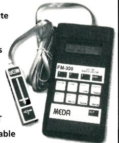
Our single and three axes handheld fluxgate magnetometers measure weak magnetic fields from 1 nT to 200  $\mu$ T. Our FM300 Vector magnetometer has a 1 nT resolution over a  $\pm 100 \mu$ T range and can be computer controlled through an RS232 communications port.
