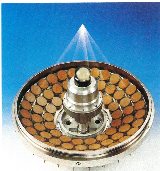
FIGURE 2. LITHOTRIPTER sound source (a) and output trace (b). a: Piezoelectric actuator head for production of high-intensity sound in a lithotripter. An array of piezoelectric sources line a parabolic dish so that the sound produced is focused on the site of a kidney stone. b: The pressure produced at the focus has an amplitude of over 1500 bars and a pulse width of about 125 nanoseconds. (Courtesy of EDAP Technomed SA, Lyon, France.)
