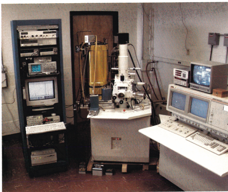
THE MICROCALORIMETER-BASED x-ray spectrometer (on left side of center table) developed by researchers at the National Institute of Standards and Technology (NIST) in Boulder, Colorado, is designed to be used with a scanning electron microscope (white) on right side of center table. The spectrometer uses an adiabatic demagnetization refrigerator (gold-colored cylinder) to reach millikelvin temperatures. The microcalorimeter is located at the end of an extension from the refrigerator, near the sample inside the SEM. The control console and signal processing electronics are located to the right and left, respectively, of the microcalorimeter/SEM assembly.
