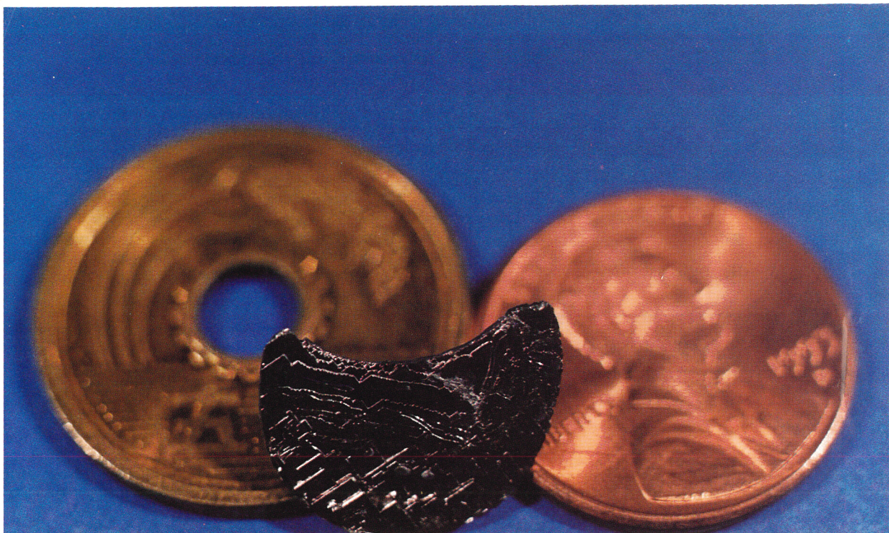
FIGURE 1. SINGLE CRYSTAL of \text{LuNi}_2\text{B}_2\text{C} grown from molten \text{Ni}_2\text{B} . The mass of this magnetic superconductor is about 1 gram.
