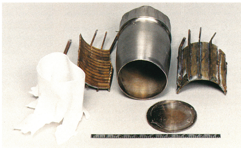
FIGURE 2. DEBRIS FROM A FATAL "cold fusion" cell explosion that occurred in a Menlo Park, California, electrochemistry laboratory on 2 January 1992. Shown are the main stainless steel electrolysis cell and its detached base, a ripped Teflon insert and pieces of brass heat-exchanger fins.
