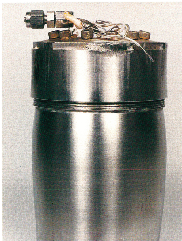
FIGURE 3. SIDE VIEW of the main “cold fusion” vessel that exploded accidentally in a Menlo Park, California, electrochemistry laboratory on 2 January 1992. Note the bulge below the metal threads. An increase in internal pressure prior to the explosion deformed the 0.2 cm thick, stainless steel cell from an initial configuration of a right-circular cylinder.
