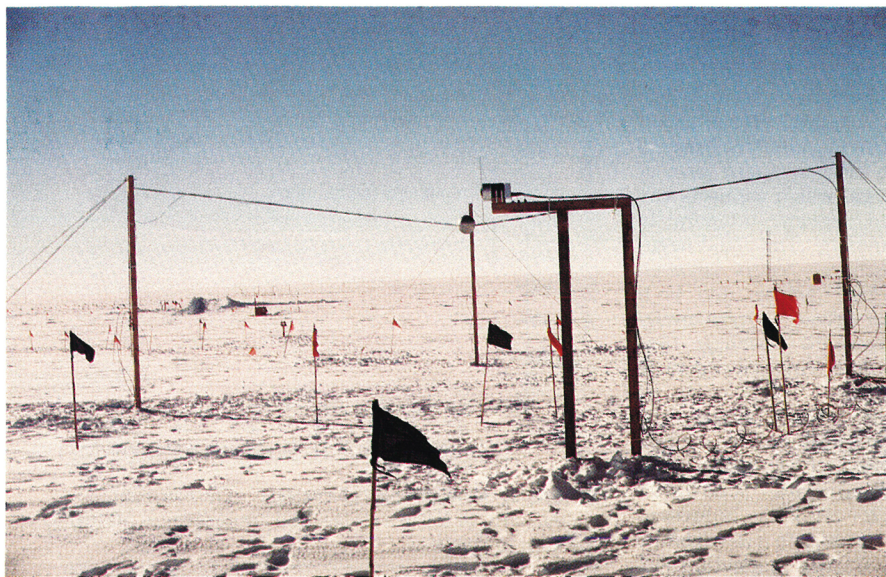
FIGURE 5. CURRENT AND FIELD SENSORS at site 1 near South Pole Station, 15 January 1991. The sphere is an air-Earth atmospheric current sensor. The 17.8 cm split sphere, located about 4 m above the snow, contains a differential ammeter for measuring the difference in current flowing to the two hemispheres. The device on the framework in the foreground is an electric field sensor. It is a vertically oriented 30 cm dipole electric-field mill about 3 m above the snow surface. (Photo by Gregory J. Byrne, copyright 1993 American Geophysical Union, reproduced with permission.)
