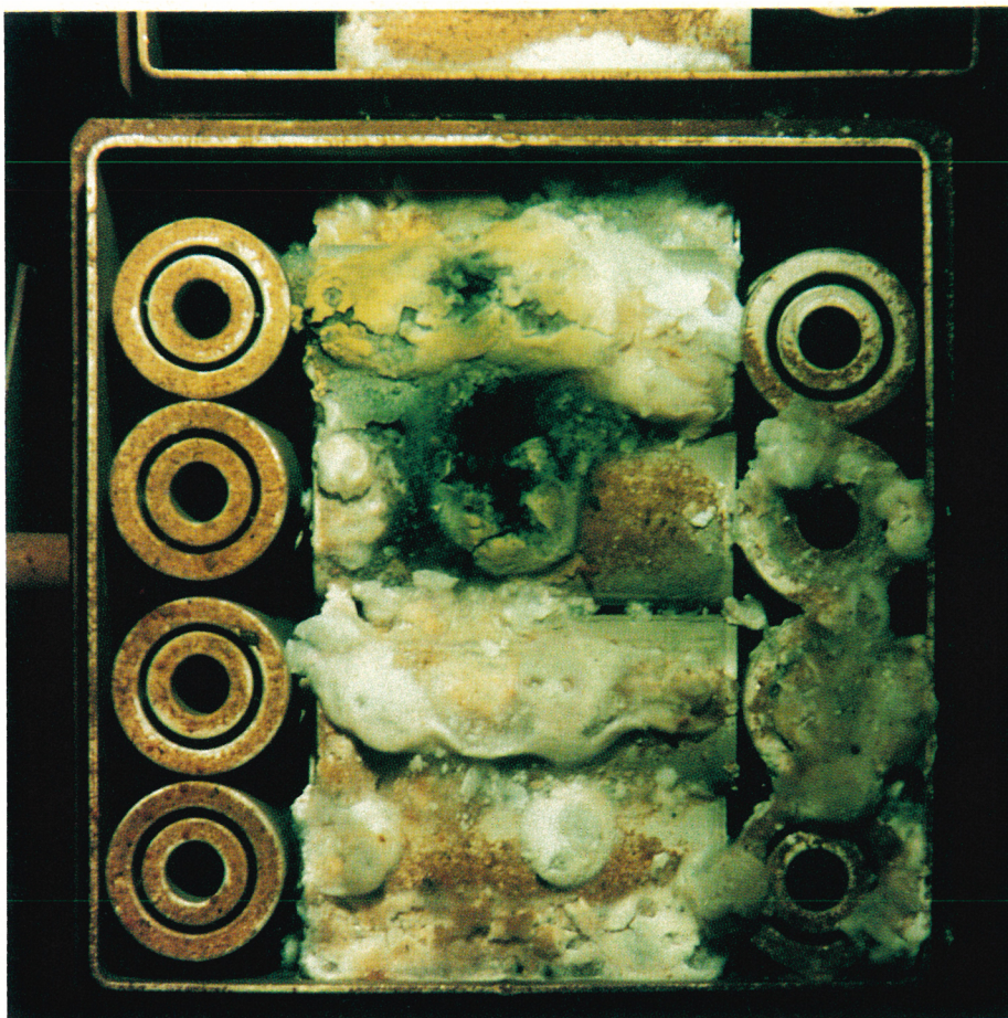
CORRODED PLUTONIUM-BEARING FUEL TARGETS from a Savannah River reactor formerly used to make plutonium-239 for weapons. These targets, 4 inches in diameter and 14 inches long, have since been converted to a stable metal form for long-term storage.
