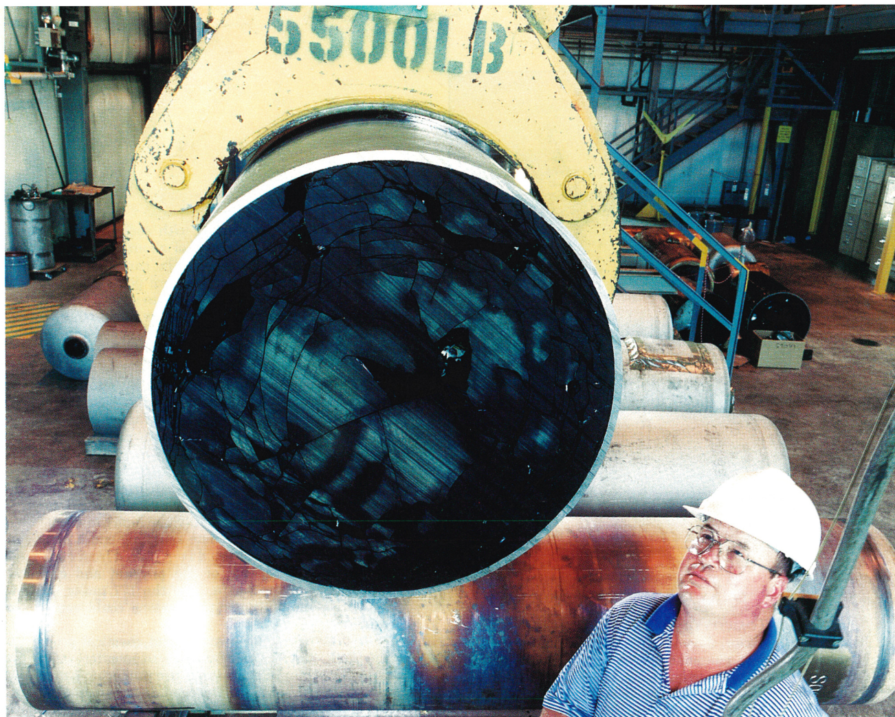
FIGURE 1. GLASS CANISTERS AT SAVANNAH RIVER. Reprocessing waste is being incorporated into borosilicate glass at the Defense Waste Processing Facility at the Department of Energy's Savannah River site, near Aiken, South Carolina. Before the facility went "hot" in 1996, a test run was made in which 80 canisters were produced by pouring molten glass into cylindrical stainless steel containers using nonradioactive materials to simulate the properties of the waste. The canisters are about 3 m high and about 0.6 m wide and contain about 1700 kg of glass when filled. In the test canister visible in cross section, note the concentric fracture pattern formed during cooling. (Photo courtesy of Westinghouse Savannah River Co.)
