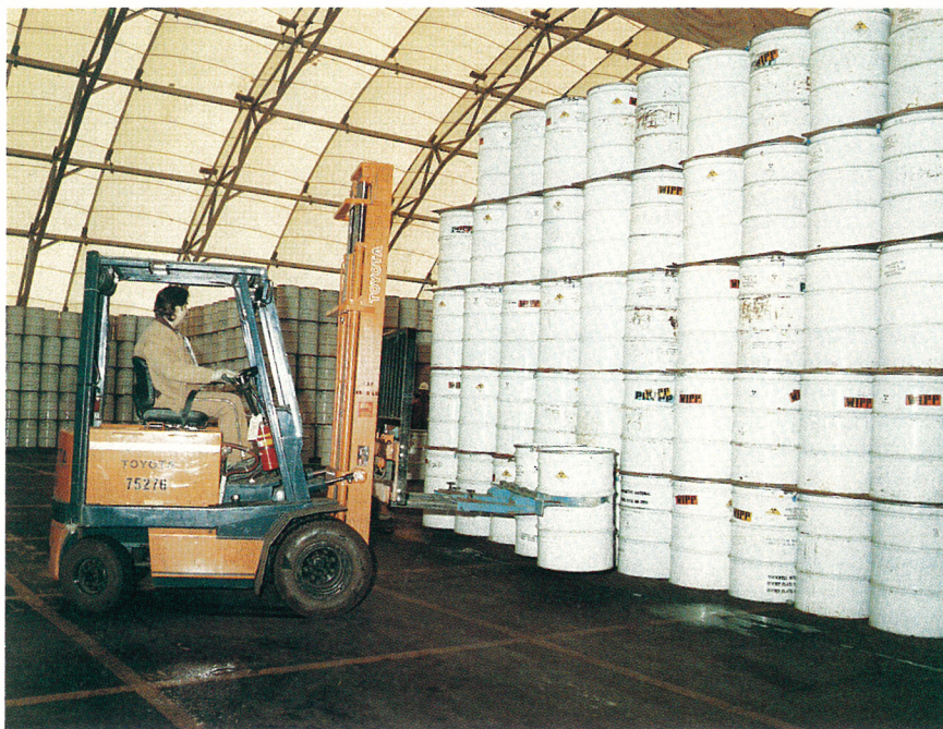
FIGURE 4. BARRELS OF TRU WASTE being stacked in a building at the Idaho National Engineering Laboratory. DOE is studying the suitability of long-term disposal of such wastes at the Waste Isolation Pilot Plant in New Mexico. (Photo courtesy of DOE.)
