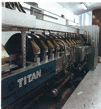
e^-e^+ Injector for DAΦNE at INFN, Frascati, Italy. Recent Results: 535 MeV, 32 ma positrons.
